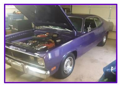
• Currently powered by a High Output 318 V8.
